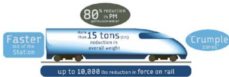
locomotive weight by more than 15 tons. These lighter-weight locomotives will accelerate and decelerate faster, allowing
